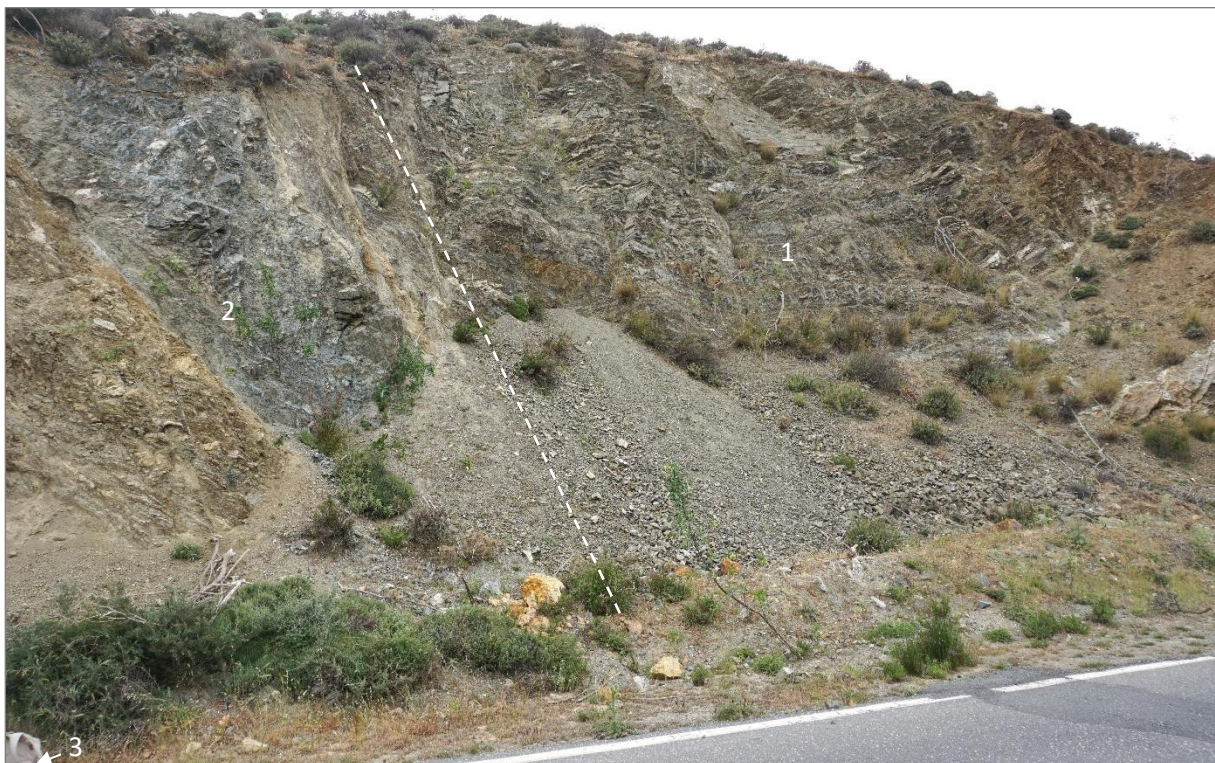
Outcrop I: Country rock and fault zone next to the serpentinite body. 1: undisturbed calc-silicate schist
