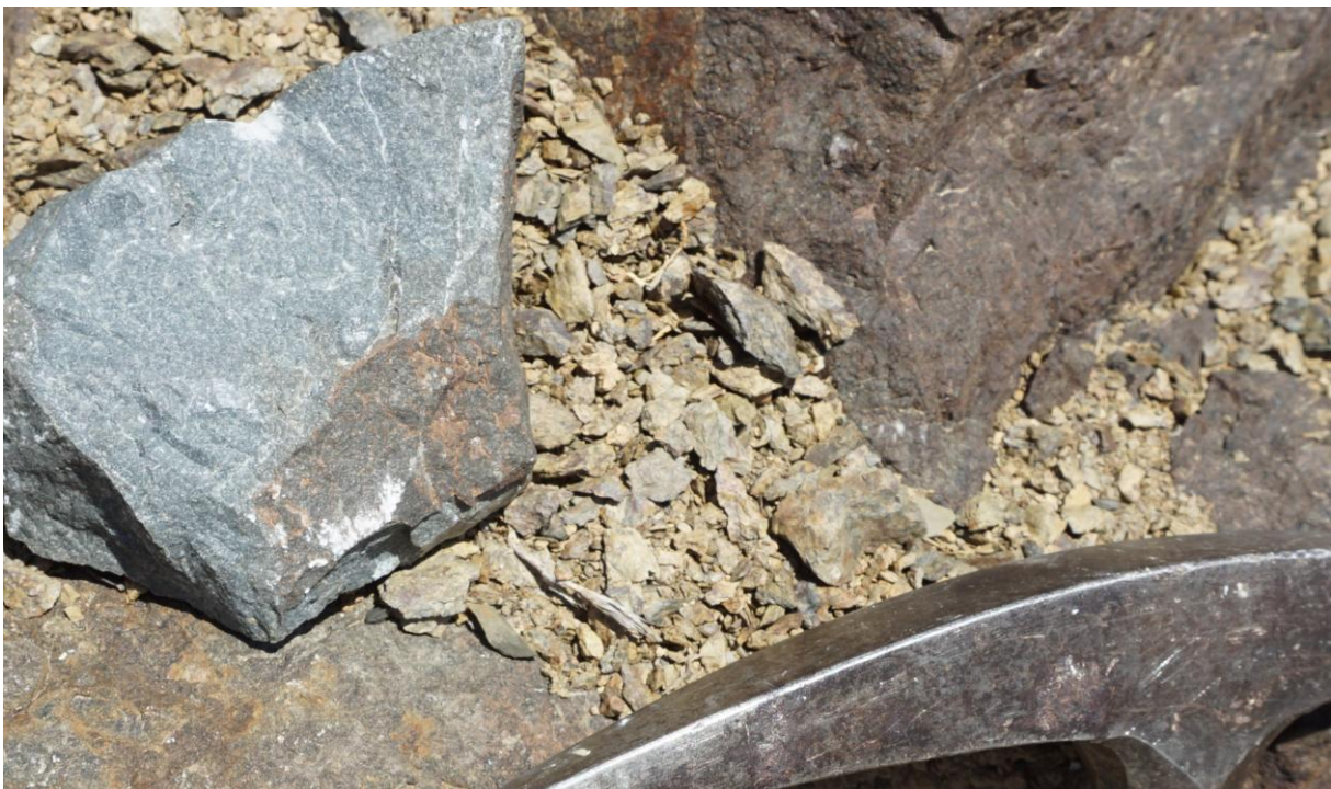
Outcrop V, close up showing weathered and fresh rock surfaces. The light grey colour indicates the rock to be of andesite composition.
