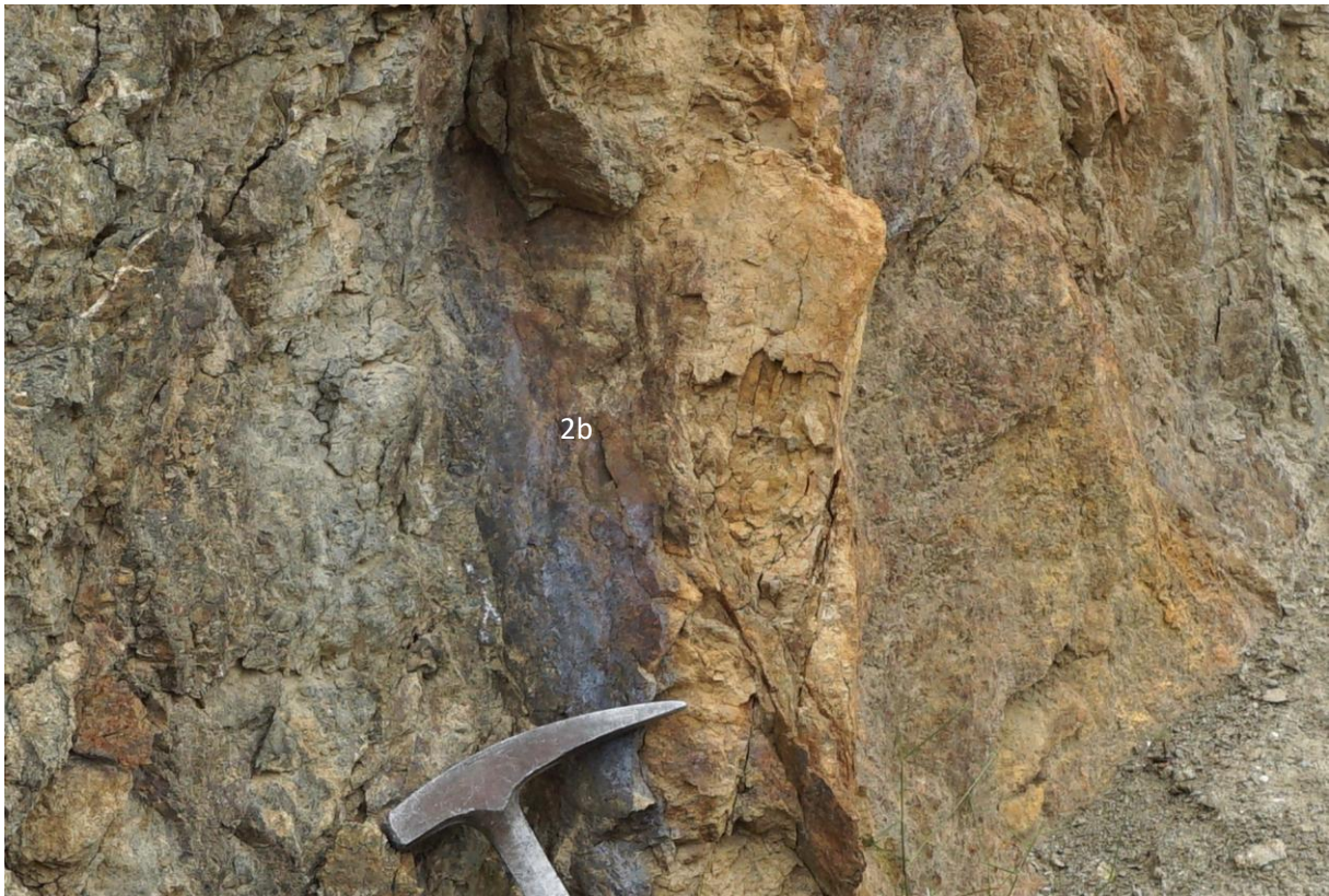
Outcrop I, 2b: hydrothermal vein displaying metal deposits (iron ?). Orange gangue rock could be former mafic /ultramafic rock.
